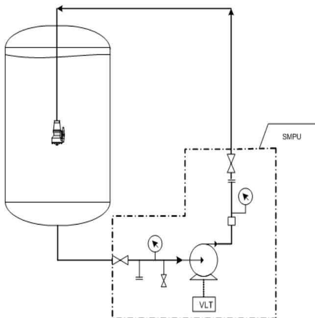
The unit contains an Alfa Laval centrifugal pump with suitable frequency converter piping, two pressure gauges, two manual valves at inlet and outlet plus a drain valve. An instrument house prepares the unit for potential installation of instrumentation.
