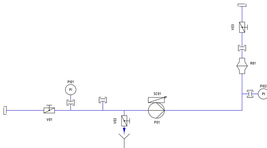
On the suction side of the pump there is a manual butterfly valve, a pressure gauge and a blind connection plus a drain.
