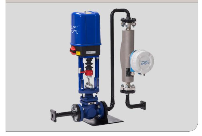
The Coriolis flow meter (CFM) upgrade kit contains everything needed to replace the spindle flow meter in your Alfa Laval Aalborg burner with a Coriolis flow meter. Based on the Coriolis principle, this type of meter is a simple and highly accurate solution without any moving parts. Performing the upgrade ensures more durable boiler equipment that is line with today's standards.
